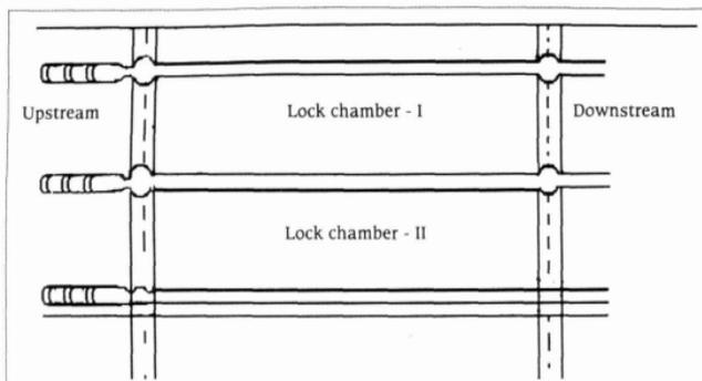
Fig. 4 : Diagrammatic representation of two lock chambers of fish lock in Farrakka Barrage
