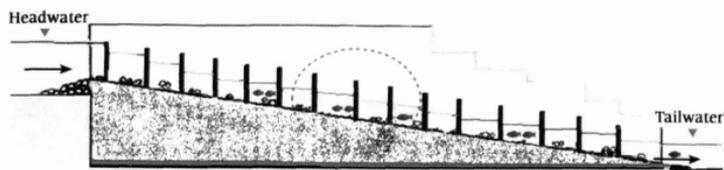
Fig. 1 : Diagrammatic representation of a conventional pool pass (After Jens 1982, DVWK 2002)
