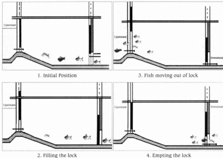
Fig. 5 : Operation of fish lock at Farrakka Barrage (Diagrammatic representation)
