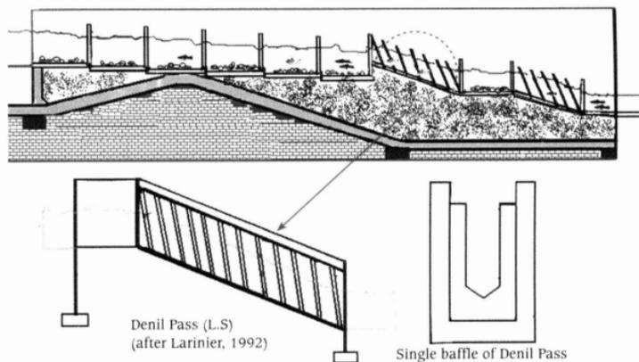
Fig. 2 : Diagrammatic representation of Denil type fish pass in Naraj Barrage (Modified, source, Das 2002)
