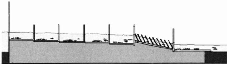
Fig. 3 : Diagrammatic representation of Denil type fish pass in Hathnikund Barrage (Modified, source, Das 2002)
